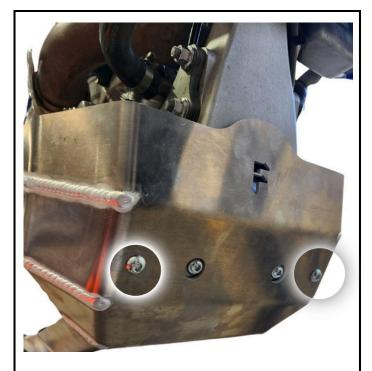
POSITION bash plate up to U-clamps and INSERT 2x M8x20 Button Head bolts through the bash plate and into the mounting pate. PUSH bash plate hard up against frame, then tighten.
