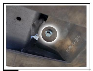
INSERT 1x M6x16 Bolt through rear of Bash Plate and TIGHTEN
