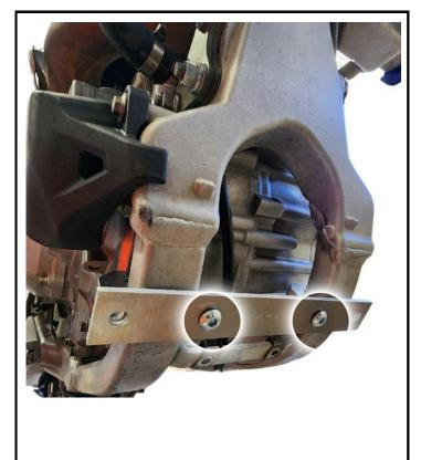
Using 2x M8x16 button head bolts, SECURE the mounting pate to the U-Clamps
