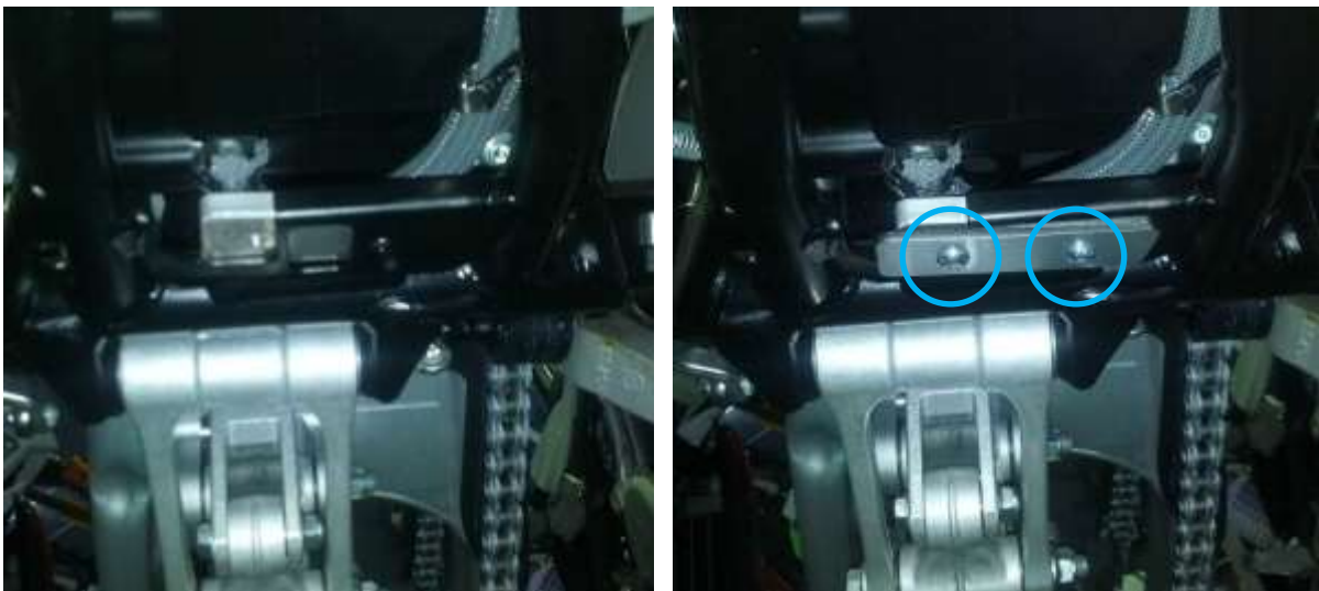
Figure 2 - Mounting of underside blocks
