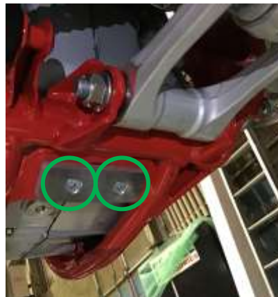
Figure 4: Place the 8mm alloy block (hq-03-f) on the top of the frame and (Hq-03-G) to the bottom of the frame and fasten with provided flathead bolts.
