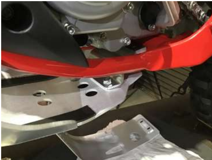
Figure 5: Slide bash plate over the aluminium blocks (from figure 4) that are mounted to the frame
