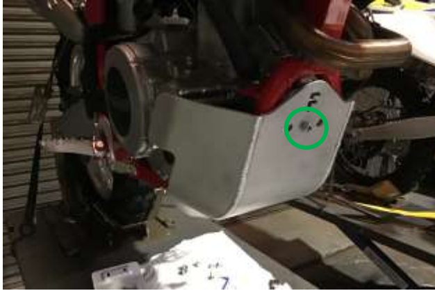
Figure 6: Tighten the front bolt with 6mm Allen Key
