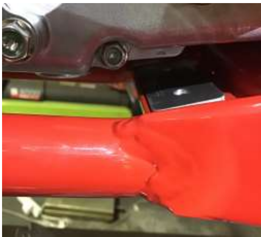
Figure 4: Place the 8mm alloy block (hq-03-f) on the top of the frame and (Hq-03-G) to the bottom of the frame and fasten with provided flathead bolts.
