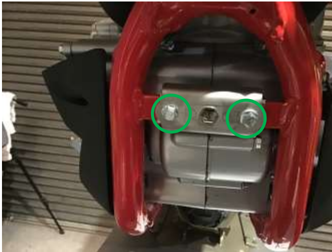
Figure 3: Place the Front Bracket (HQ-03) to the bike and mount with the supplied bolts
