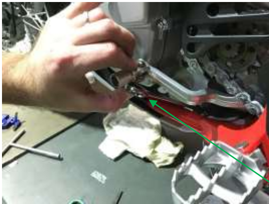
Figure 7: Tighten the rear bolts as shown with 13mm spanner
