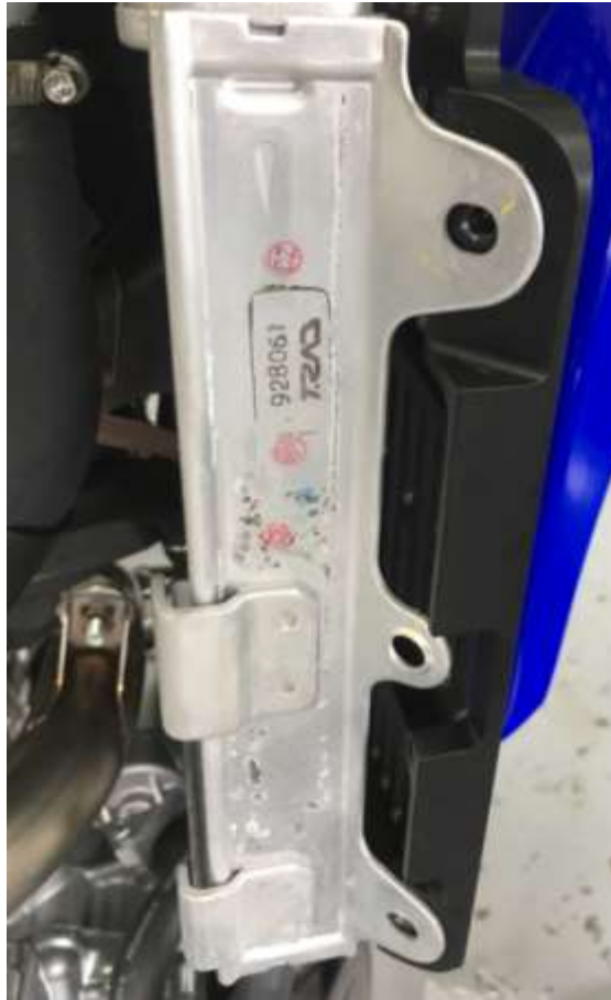
Figure 3: Fitted guard, ready for the radiator shroud to go back on
