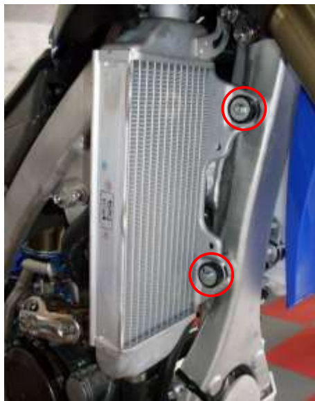
Figure 2: Radiator shrouds removed
