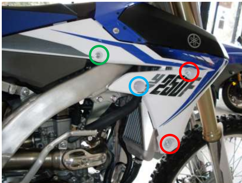
Figure 4: Refitting the radiator shrouds
