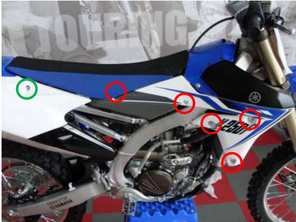
Figure 1: Mounting bolts for the seat and radiator shrouds
