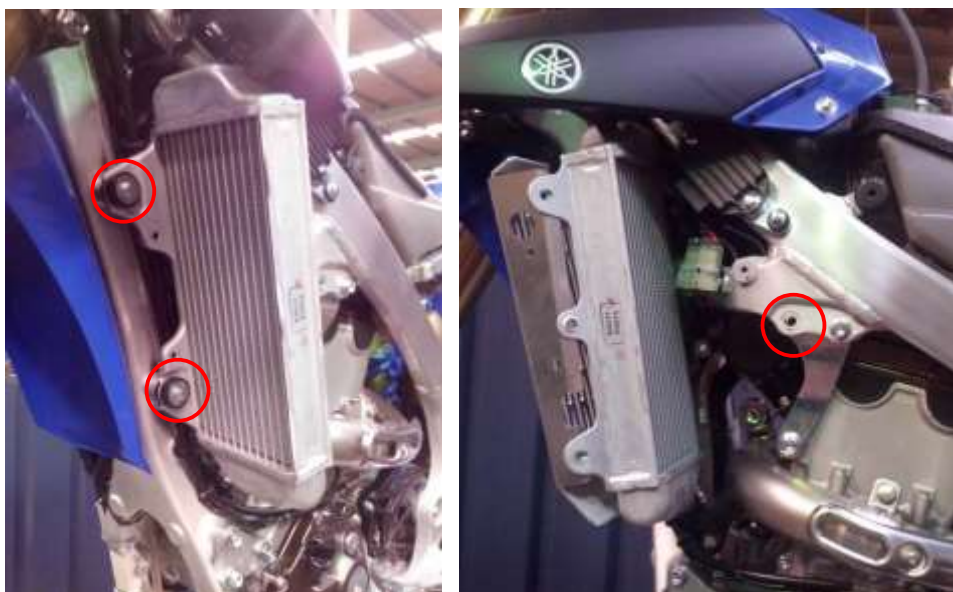
Figure 2: Radiator shrouds and engine mount bolts removed
