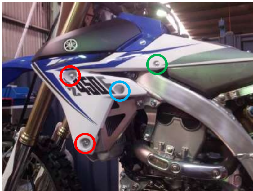
Figure 4: Refitting the radiator shrouds
