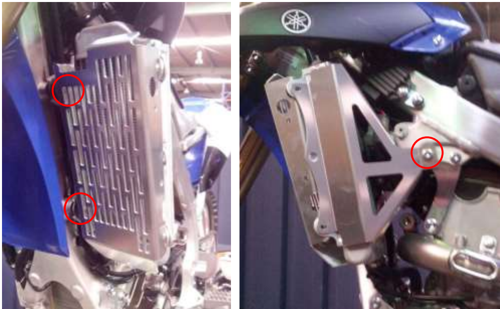
Figure 3: Fitted guards and braces, ready for the radiator shrouds to go back on
