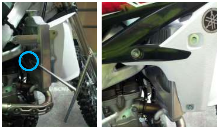
Figure 2: Fitting the brace and refitting of fairings (From left to right; a & b)
