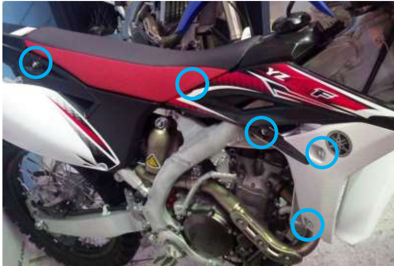
Figure 1: Mounting bolts for the seat and fairings
