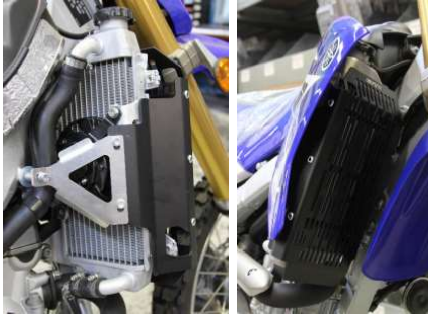
Figure 3: Fitted guard and brace
