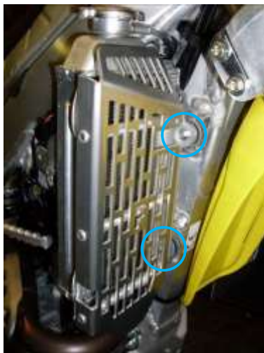
Figure 2: Fitting radiator guards and clamps (From left to right; a, b & c)
