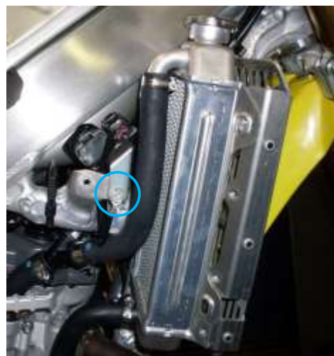
Figure 2: Fitting radiator guards and clamps (From left to right; a, b & c)
