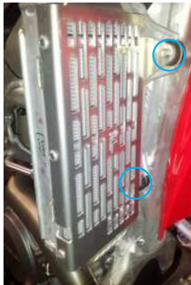
Figure 2: Fitting radiator guards
